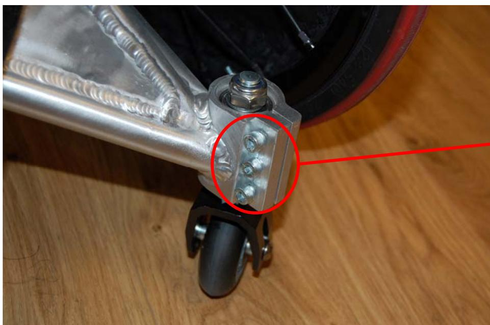
Using a 6mm allen key simply slacken 3 allen screws, slide inner socket up or down to set height and retighten
